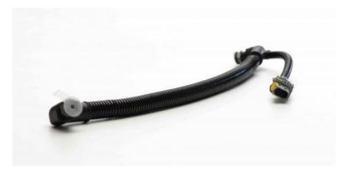
Our heated SCR line links the tank to the injection system on the exhaust line, supplying it with AdBlue® fluid. Our solution, created exclusively with thermoset thermoplastic materials, is lightweight and easy to install. Its heating power can be tailored to each customer's needs thanks to the smart choice of integrated resistant wires in the line wall.
