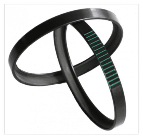
Hutchinson develops standard or customized magnet rings, made of a metal insert bonded together with a rubber matrix filled with magnetic particles. The elastic properties of the rubber, combined with good rubber-metal adhesion, ensure good performance under extreme environments. We customize magnet rings to fit perfectly to various technologies of sensor such as Hall Effect, AMR or GMR...
