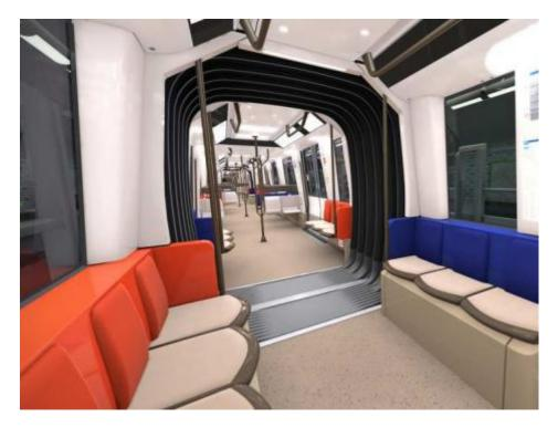
Our Inter-Vehicle Gangway solution allows passengers to walk safely from one car to the next on trains and tramways. It offers high-performance soundproofing, protection against fires and is ideal for intensive use.
