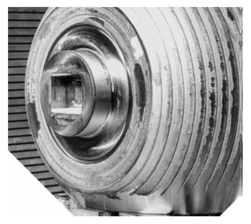
Cladded balls from design to manufacturing, following Welding Procedure Specification, prepared according to our worldwide customer's requirements. The welding overlay is obtained by depositing on a base material surface, usually carbon steel, two or more layers of protective material.
