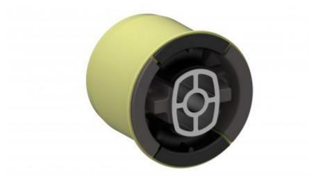
Our Dual Compound Bush is a solution for the rear axle twist beam. Thanks to the stiff rubber used in the horizontal axis and the low dynamic stiffness in the vertical axis, it enhances passenger comfort. It offers a performance between conventional and hydrobush solutions. It is designed to dampen vibrations from the road and absorb shocks. It plays a key role in improving vehicle performance, safety and passenger comfort.
