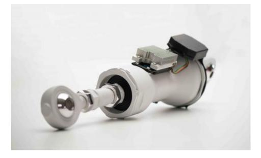
With our Embedded Health and Usuage Monitoring System, sensors mounted on frequency adaptors for helicopters monitor displacement, force, pressure and temperature. Data are analyzed and stored in flight, allowing the component's health to be assessed and data on real operating conditions to be saved.
