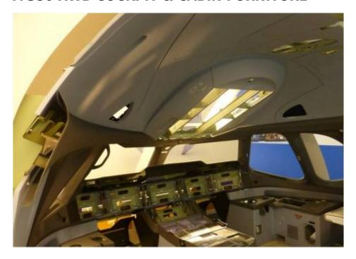
Our wide range of products includes panels, cabin interior structures and tailor made solutions for commercial, business jets and VIP aircrafts. We design, manufacture and deliver ready-to-install cockpit and cabin kits directly onto the aircraft, incorporating all the options defined in the agreement with the customer.
