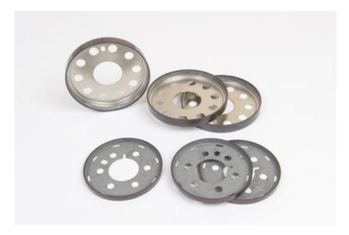
Our magnet ring for engines determines very precise measurements of the position and the rotation speed of the crankshaft or the camshaft. They transmit an accurate and optimized input signal to the electronic control thanks to the sensor. Our solution pinpoints the precise position of the top dead center of the engine, helping carmakers improve their Stop & Start systems and fuel injection management.
