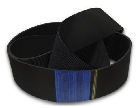
Our solution transmits power from the engine to the oil pumps, withstanding pump torque and motor loads. Our On Shore Poly V<sup>®</sup> belt is a power transmission belt that features multiple longitudinal ribs. The molding process ensures an optimal quality. The contact of the belt rib flanks and the pulley grooves transmits the torque. Thanks to custom-developed materials, our On Shore Poly V<sup>®</sup> belts are resistant to both high and low temperatures, dynamic loads and abrasion.
