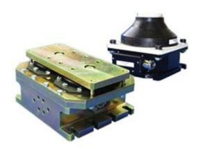
Our active noise and vibrations control system  $\mathsf{STRACTIVE}^\mathsf{TM}$  cancels incoming vibrations by generating a dynamic force of the same magnitude in opposite phase through the use of electrodynamic actuators. It improves vibration insulation in the range of 10 to 1.000 Hz (-12 to -36 db).
